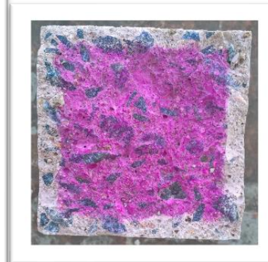
Carbonation depth measurement
